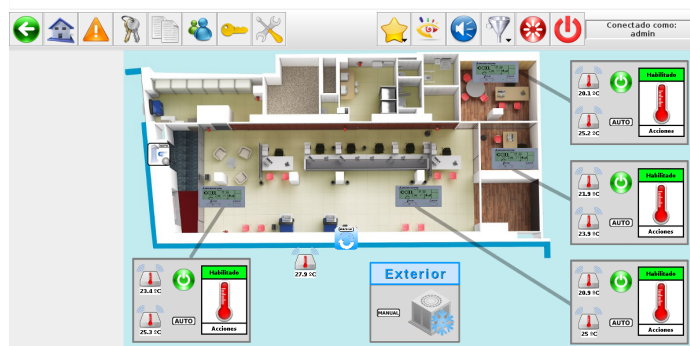
(a) SCADA-web view showing some HVAC automation actions
