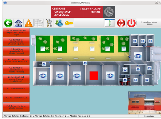
Figure 5 SCADA-web view of the ground floor of the reference smart building
